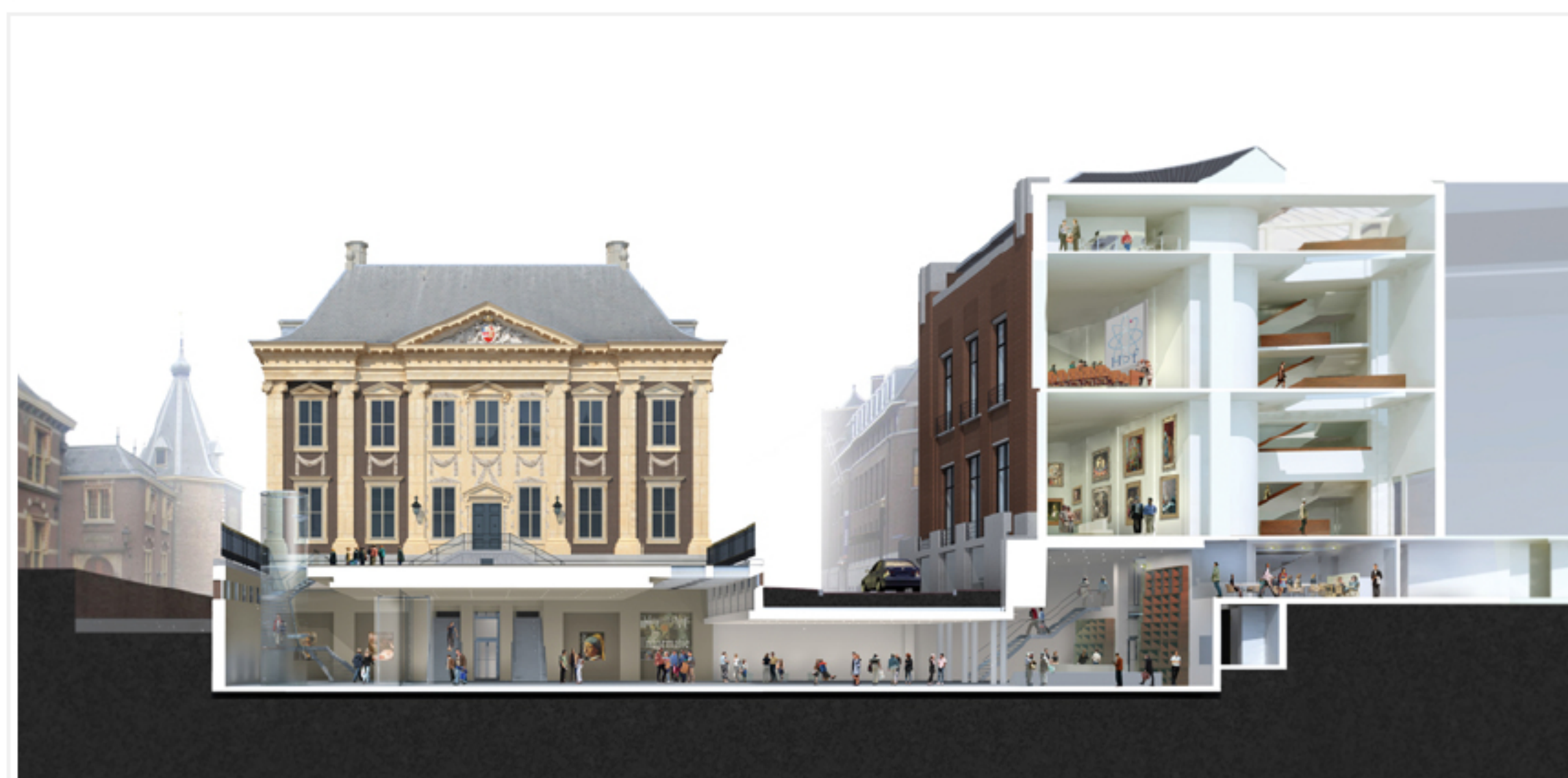
A section shows the connection between the existing museum and an addition occupying the building across the street.
